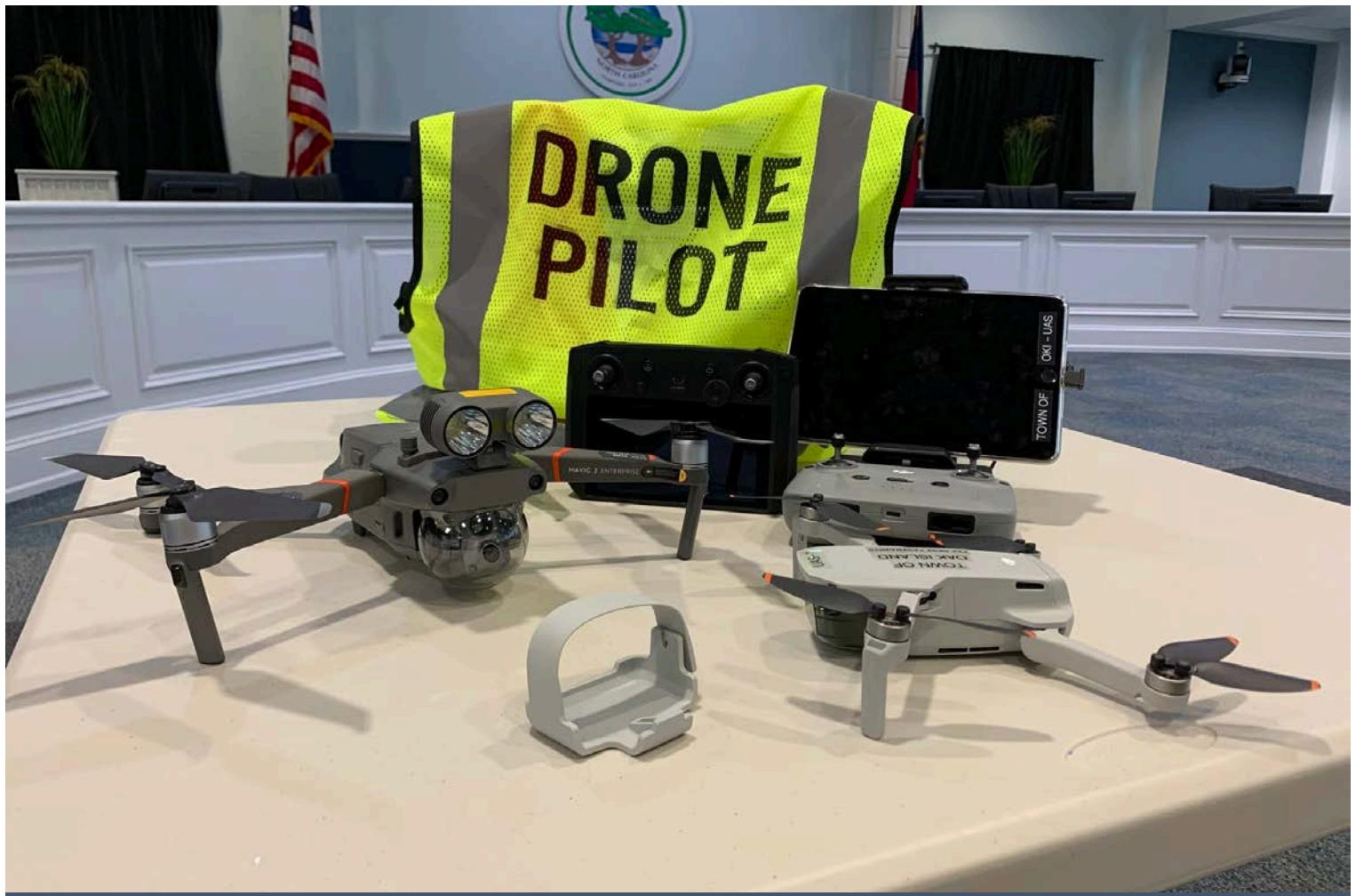
**EQUIPMENT PROFILE:** *Mavic II Enterprise Advanced: (pictured left)* is the pinnacle of lightweight performance, packed with extreme capability. Manufactured by DJI, the industry standard in commercial drones, the Mavic II joined as the flagship of the Oak Island fleet at the end of April.
