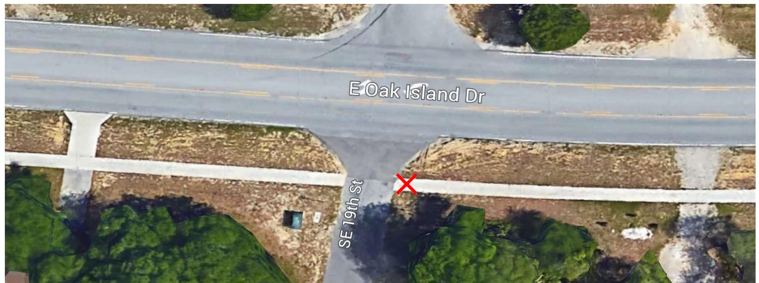
**X** = Remove and replace existing sidewalk, add a raised truncated dome.
