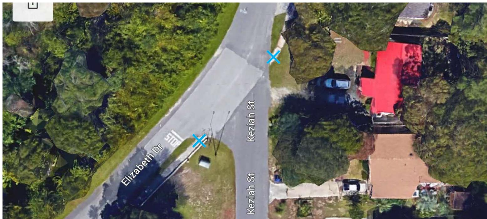
**X** = Remove and replace existing sidewalk, add a raised truncated dome. (See note)
