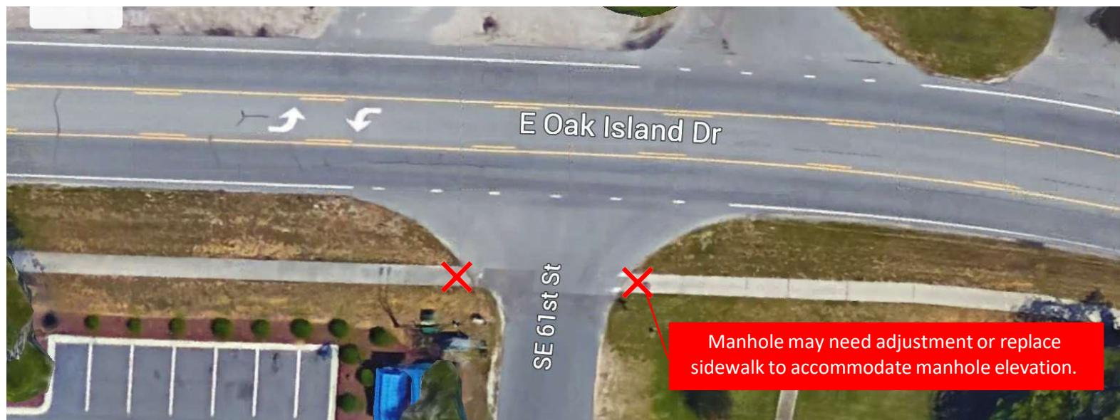
**X** = Remove and replace existing sidewalk, add a raised truncated dome. (See note)
