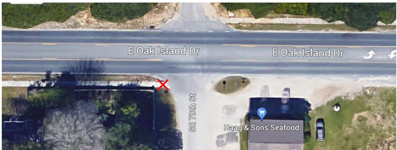
**X** = Remove and replace existing sidewalk, add a raised truncated dome.
