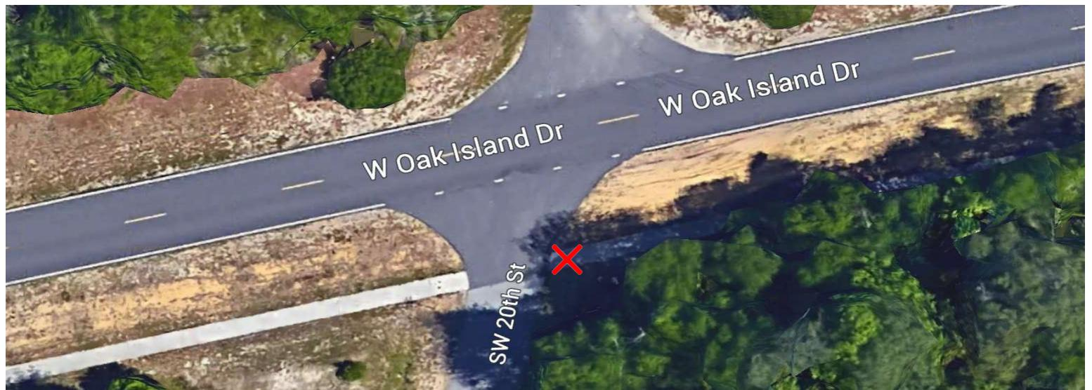
**X** = Remove and replace existing sidewalk, add a raised truncated dome.
