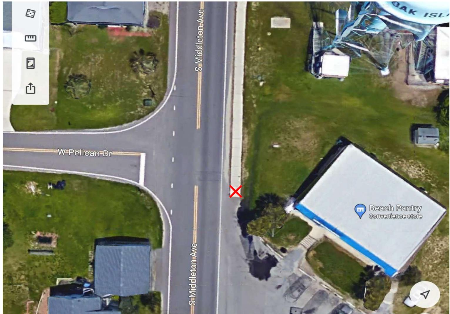
**X** = Remove and replace existing sidewalk, add a raised truncated dome.
